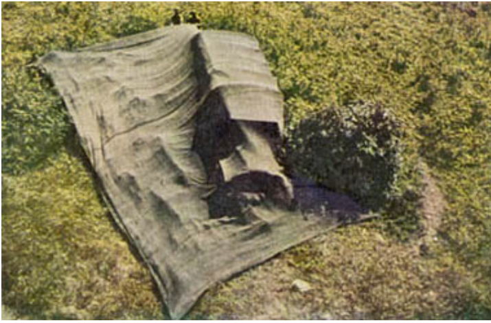
FIGURE 49 (c) and (d). In upper picture, drape is unrolled over vehicle; ends are spread out and partially staked down. More of net is on the shady side, stretching out farther with a gradual slope. Draping must not stop at this stage. Below, poles prop net off top of vehicle, creating an irregular shape. Addition of small branches completes the job.
